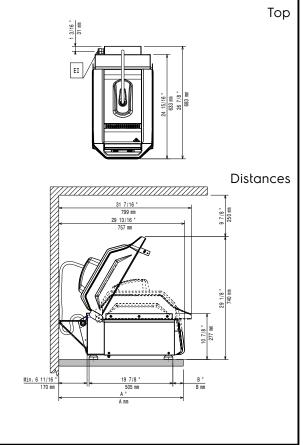
Plug In SpeeDelight with adjustable tube, ribbed, removable teflon plate, 5kW 230V The company reserves the right to make modifications to the products without prior notice. All information correct at time of printing.
